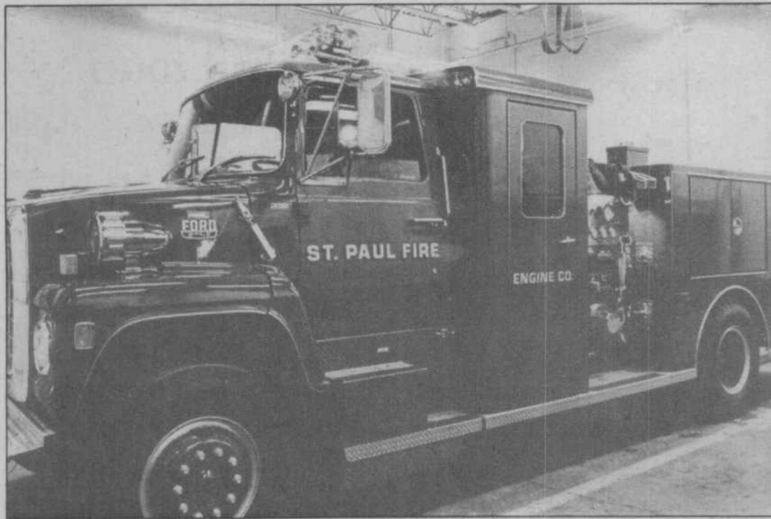
Fire station number 23, serving St. Anthony Park, has just received a new Ford diesel pumper. This new truck carries 500 gallons of water and can pump 1,000 gallons of water per minute from streetside hydrants. In addition to 2,600 feet of hose, the truck can carry four people inside, so firefighters can arrive at a fire ready for action no matter what the weather is like. With a 15 foot, 8 inch wheelbase, the truck is more maneuverable in the narrow streets of St. Anthony Park. The new truck was necessary because many parts were no longer available for the station's 1955 International pumper. Photo by Jon Madsen
